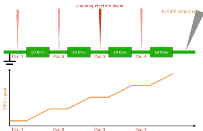
Fig. 1: EBIV signal generation principle. The electrons delivered by the scanning electron beam (red) flow to ground (bottom left) and induce a potential drop.
