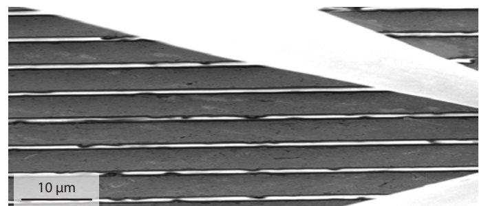
Fig. 9: Four-point resistance measurement yielding a resistance of 1.07 \text{ Ohm} across the FIB cut.
