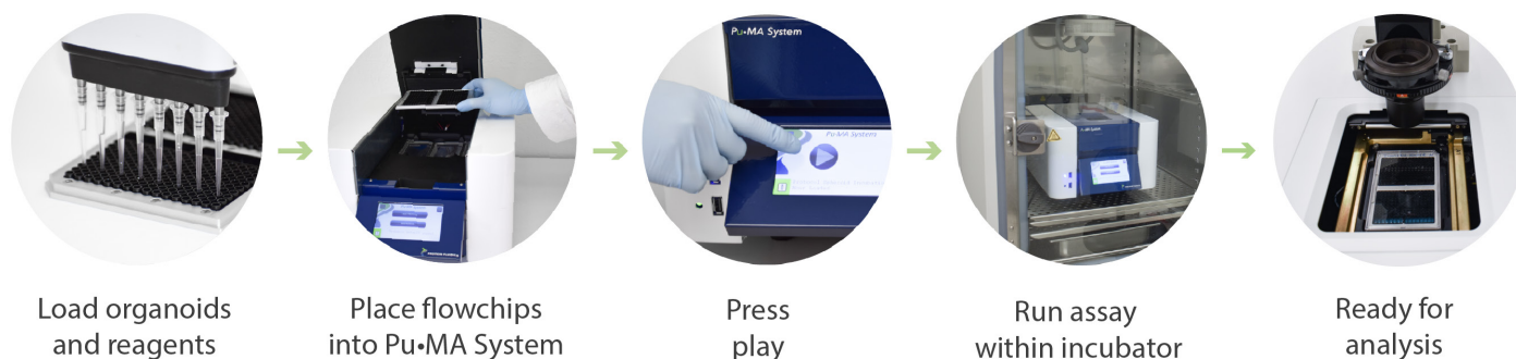
Figure 1. Schematic of the Pu·MA System workflow for automated organoid assays, in situ staining and imaging.
