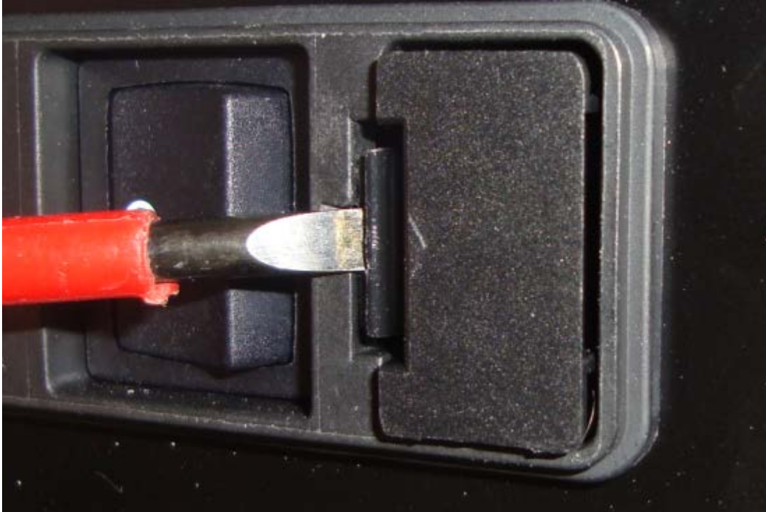
Figure 29: Mains fuse holder removal
