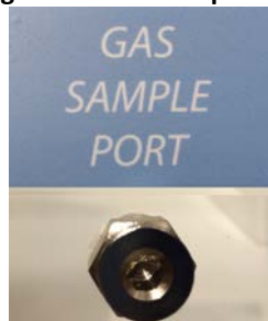
Figure 23: Gas Sample Port
