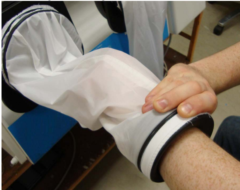
Figure 15: Entering the cuffs of the Ezee Sleeves
