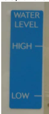
Figure 25: Pressure relief/ humidifier tank level indicator
